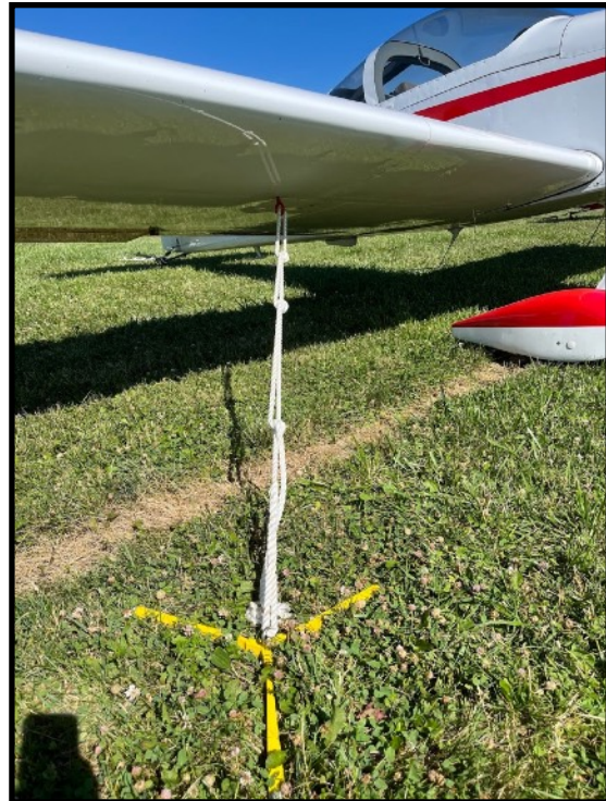
With so many priceless, irreplaceable airplanes at OSH, 3 contact multi-point tie-down systems are preferred!
