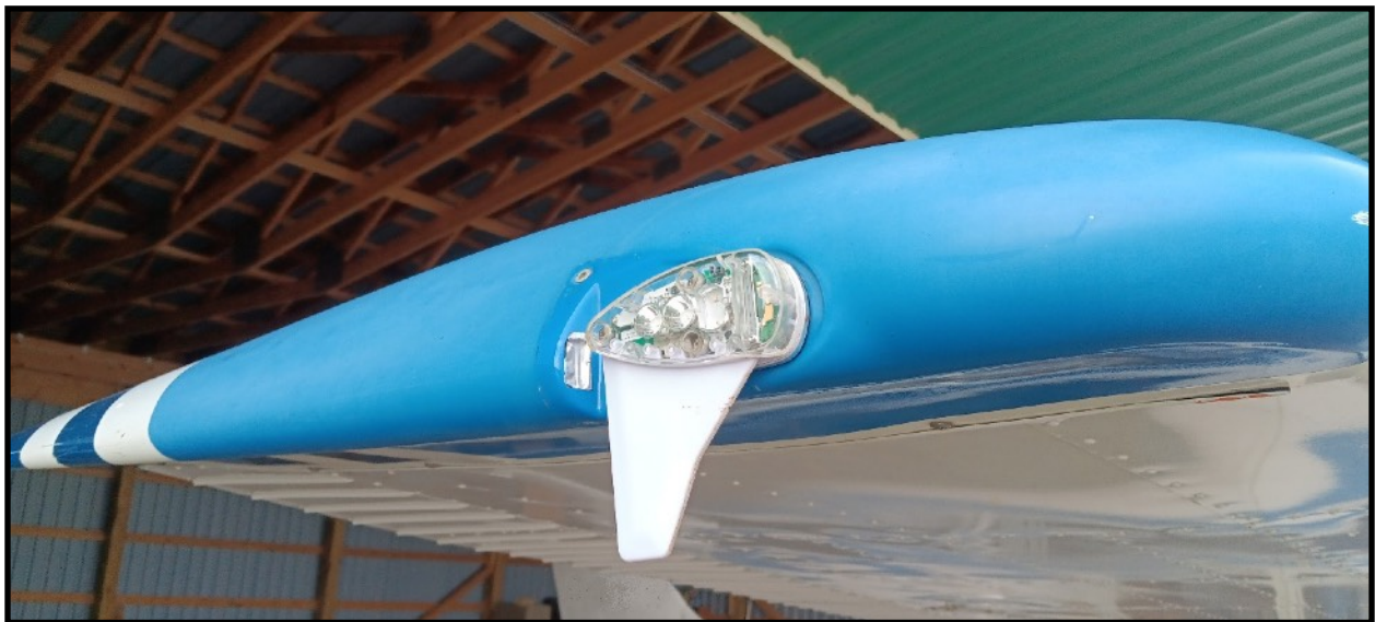
skySensor with UAT/1090 ADS-B in with GPS (plus green nav light with white strobe).
