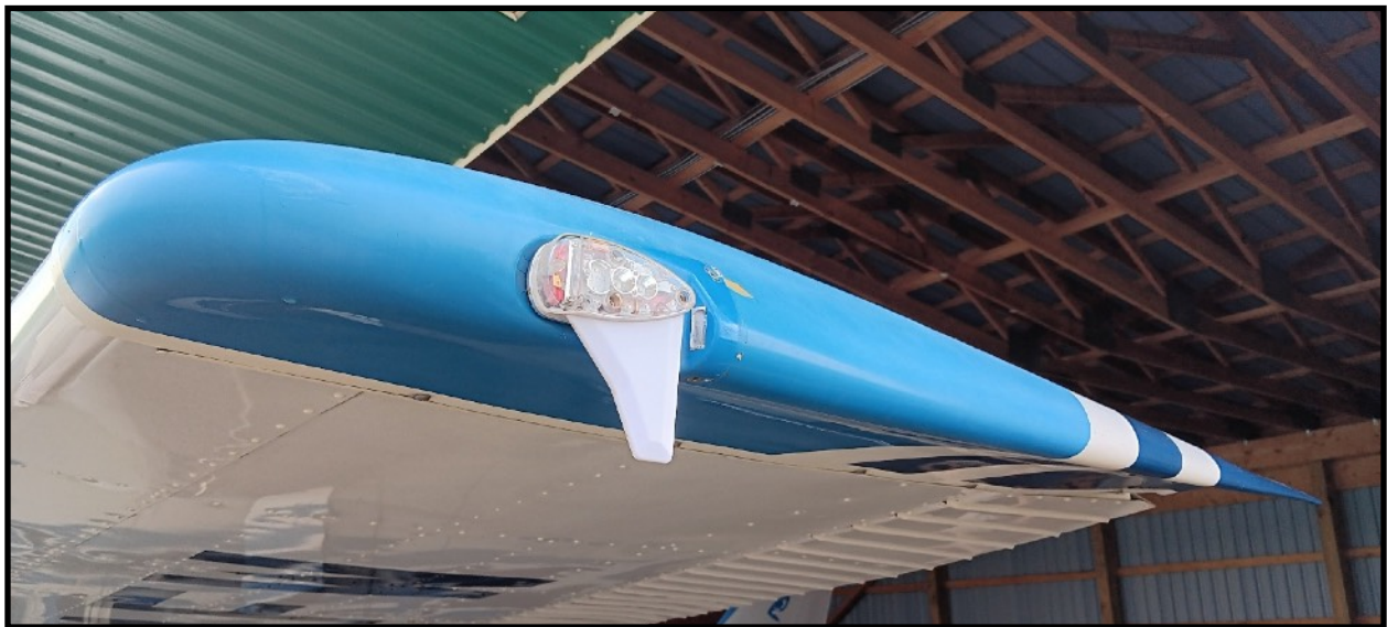
SkyBeacon on the Port Wing with UAT transmitter/GPS (plus red nav light & white strobe).
